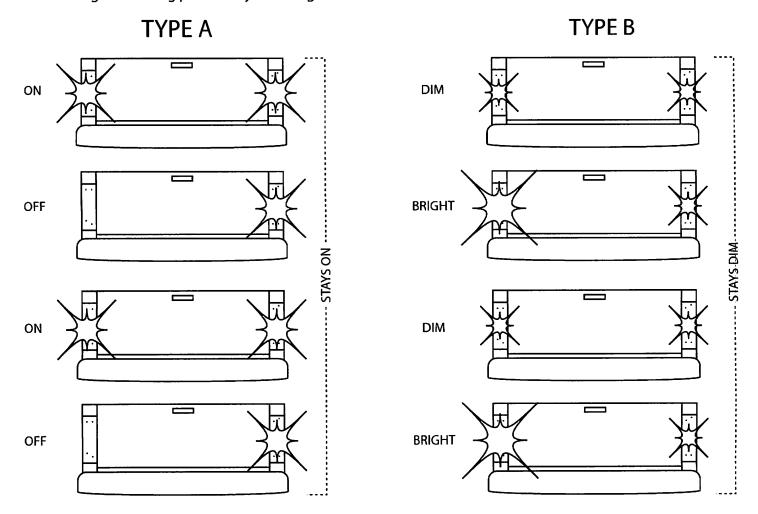
If you have Type A tail lights, your tail lights are identical to those on a trailer that uses a 4-pin Trailer Plug. Connect the running lights wire to the running lights on your tail lights. Do the same for the Left and Right turn signal wires on the Flexible Fire and Ice Bar, and the brakes will take care of themselves because your truck uses the Left and Right turn signals combined to form a brake signal. Hook the ground wire up to any ground wire or directly to the metal frame.
